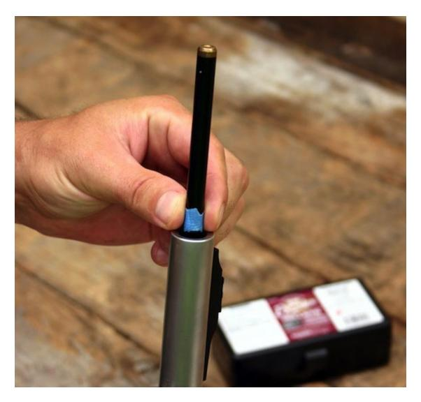
If working up loads, fully seat the bullet and mark your ramrod at the muzzle with a piece of tape. The tape is your reference point to confirm that a load is fully seated for each shot and is temporary until you find the most accurate load. Once you find the most accurate load, you can permanently mark the ramrod.
