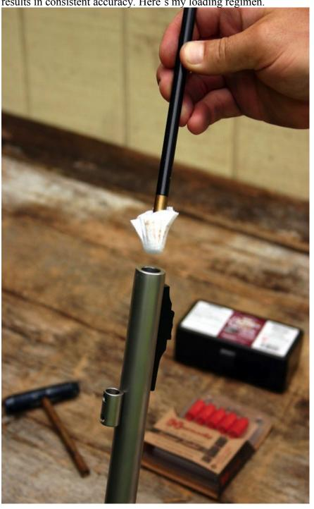
Dry all preservative oil from the bore using a clean, dry patch before loading a muzzleloader. Any residual oil in the bore can contaminate the powder resulting in hangfires or misfires and inconsistent accuracy.
