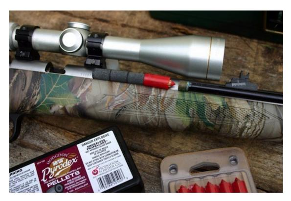
If using a load for the first time, line up all of the components on the outside of the barrel to see if it looks like the load is fully seated.
