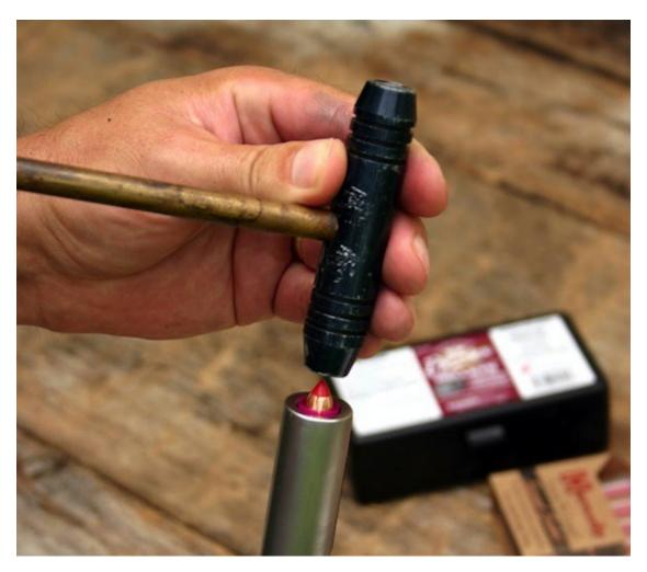
Seating bullets is a three-step process beginning with pushing the bullet just into the muzzle with a tool that fits the nose so it doesn't deform the bullet tip or start the bullet at a cocked attitude.
