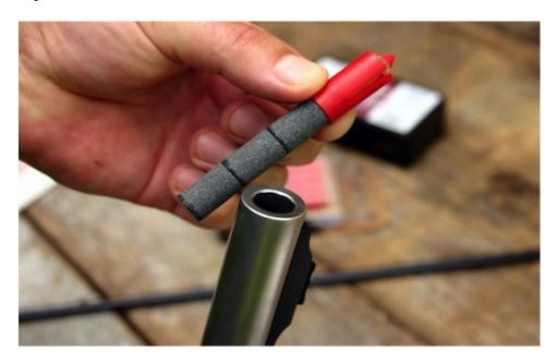
A key to accurate shooting in a muzzleloader is for the powder charge to be consistent. Loose powder should have the bullet seated with the same pressure and to the same depth for each shot. Using Pyrodex Pellets, whether used in conjunction with Hornady's Lock-N-Load Speed Sabot or on their own, is the easiest way to obtain powder consistency.
