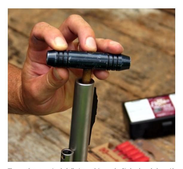
The second step to seating the bullet is to push it a couple of inches down the bore with a short starter. This step can be skipped in the field for expediency's sake, but experience shows that better shot-to-shot accuracy is obtained by using a short starter.
