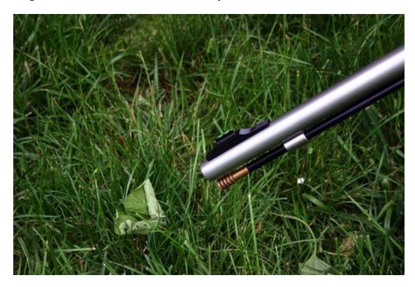
Clear the nipple for the first shot by firing a primer only in a safe direction. If you're not sure your muzzleloader is loaded, be sure to do this with the muzzle pointed toward a safe backstop. If the nipple is clear, the force of the primer should be able to move a light object such as a leaf.
