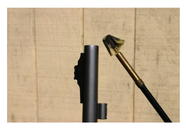
Wipe the bore between shots with a slightly moist or greased patch. This is not a thorough cleaning but simply a means of keeping powder fouling minimal, soft, and consistent.
